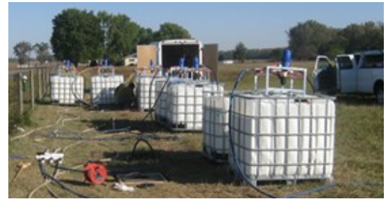
Figure 3: Dosatron® injection from totes.
