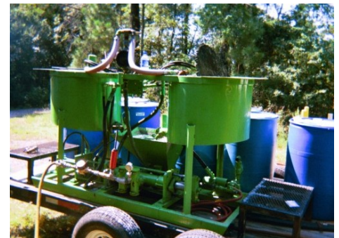
FIG. 3 — Phase II Hopper to Geoprobe
