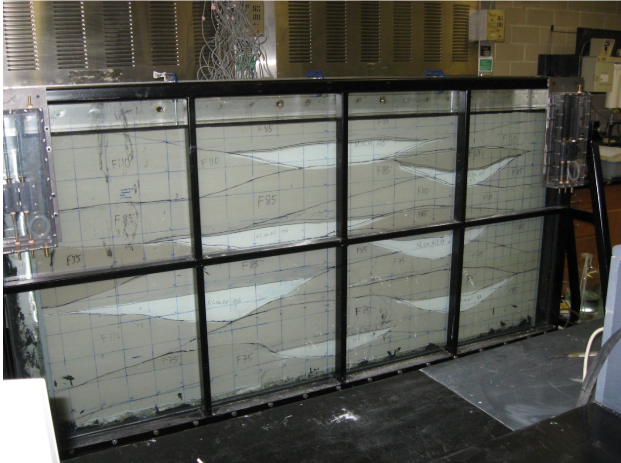
Figure 4.8.1.2: Different layers of sand and silt in the sandbox.
