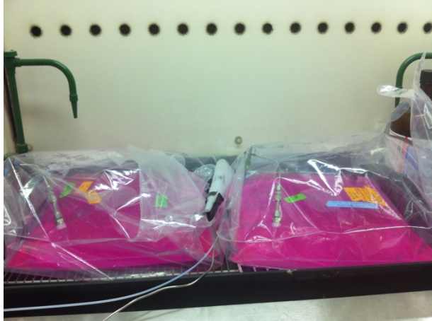
Figure 4.7.3.1: TCE source solution in The Teflon collapsible bags which are placed in glove bags.
